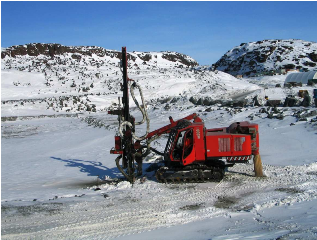
Photo 5: Drilling for thermister SRK-12-GTC-DH03
